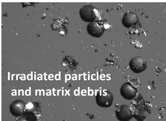
*Disintegrate matrix and liberate loose particles*
