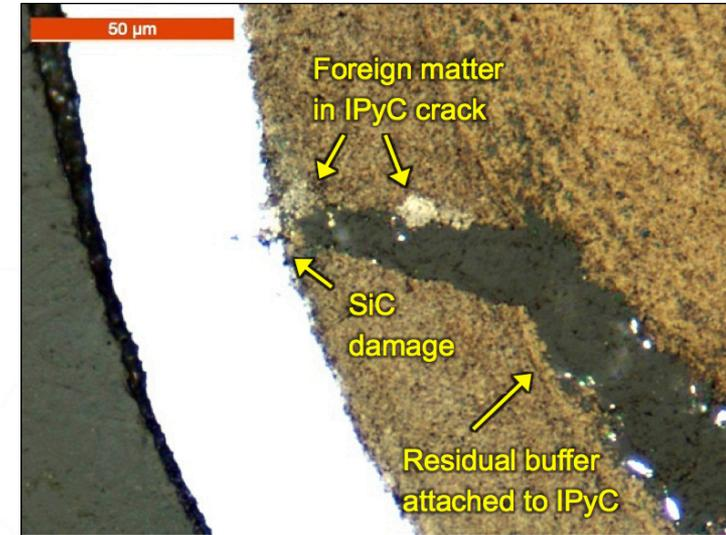
*SiC degradation and failure after 300 h at 1700°C*
