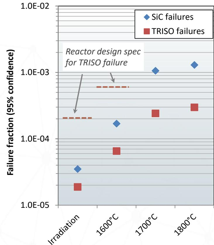
➔ AGR-1 and -2 TRISO failure fractions meet historic design specifications with ~10X margin
