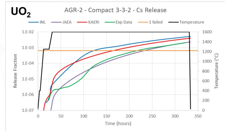
Results of computational modeling code benchmark of fission product release during high-temperature accident tests
