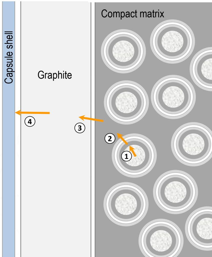
1. Release from kernel to coating layers
