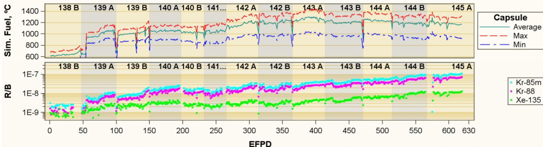
➔ *Data indicate zero as-fabricated exposed kernels or in-pile TRISO failures in this capsule*
